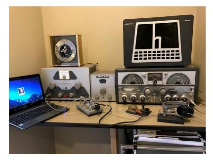
KN3DML 1958 novice station (sans VF-1). DX-40 and SX-100. (WN3R)
