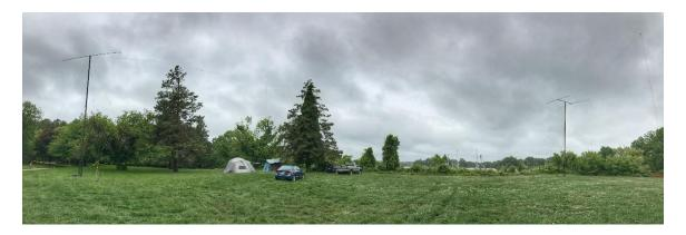
The antennas were all dipoles - 20, 17 and 15M were perched atop two 48 foot AB-577 military masts and the 80 and 40 meter dipoles were supported by 60 foot trees. Dipoles proved to be an ideal antenna choice because of Armed Forces Day activity was heavily concentrated east of the Mississippi, An eight man crew installed the all of the mast, antennas and tents in just four hours on Friday.
