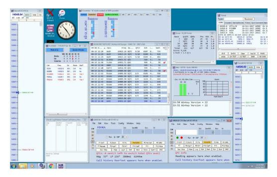
**John K3TN** – My layout on a 24" display for running SO2V1A – Single Op 2 VFOs 1 Antenna. I find that's a great mode when going gets slow in contests, as N1MM makes it very easy to work mults (or just new stations) on the right between CQs on the left.
