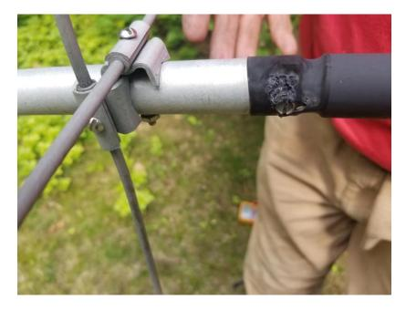
On the ground, we saw immediately what was wrong with the 40 m beam. It was what we had expected! At the end of one of the driven-element coils a stainless sheet metal screw that held the coil wire in place had loosened enough to cause a high-resistance joint. It was in plastic shrink wrap but apparently over time came loose. With high power there was arcing and scorching, quite evident once the antenna was on the ground. See the photo.
