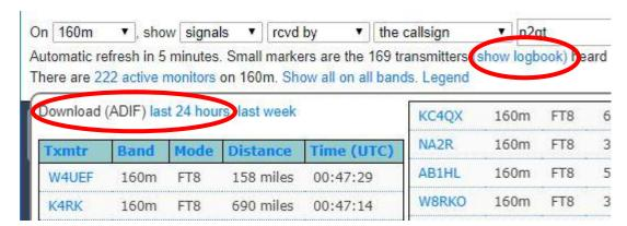
This ADIF file can then be loaded into your choice of log analysis programs. I found one on line that was designed for VHF contest log analysis that seemed to work well. Log Analyzer 3.2 found <a href="here">here</a>. On the welcome screen there is a place to specify the ADIF file you wish to analyze.
