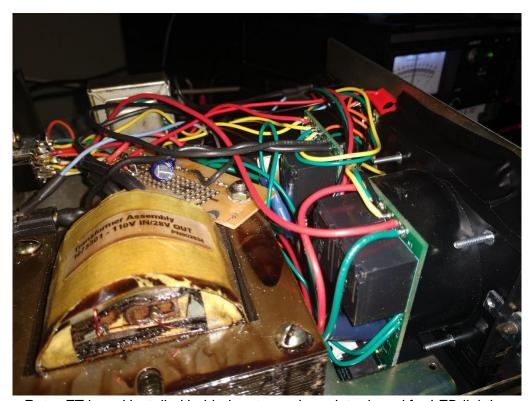
Rotor-EZ board installed behind meter and regulator board for LED lighting.
