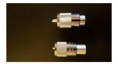
Figure 3. An Amphenol and an unmarked PL-259. The unmarked part was bought from MAX-GAIN and is known to be an excellent product.
