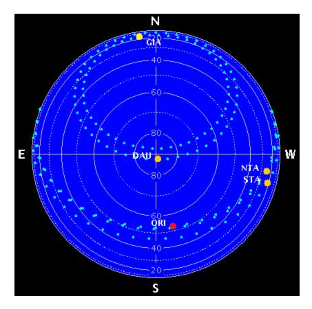
It can be easily configured to show either the path of the meteors or the best azimuth settings for your beam. With multiple showers on certain dates, using different colors, the azimuth indicator will show you the preferred direction or the path orientation of meteors dipping into the atmosphere. There is an option to only display the major showers, making the screen less cluttered.
