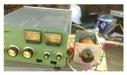
Since the amp hasn't been powered up for a while, I am bringing it slowly up to line voltage with a Variac. In the picture, I had crept it up to 56 VAC input. B+ was about 900 VDC.
