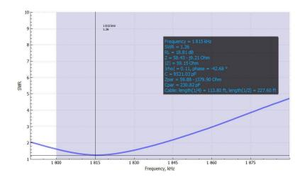
Figure 7. Inverted-L SWR.
