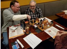
WK3A explaining his Hartley power oscillator and power supply to KW2A. The Hartley is authentic 1929 design using parallel type 27 tubes.
