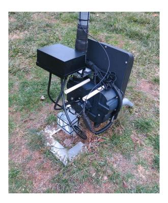
Figure 4. Steppir base with RCS-4 relay box, Balun Designs unun, and PVC standoffs . Figure 5 shows the inverted-L in place.
