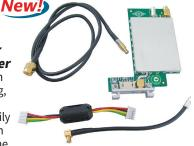
radio. This allows the use of an optional SDR receiver to provide a spectrum scope display on a much larger optional screen—without soldering and signal loss. Enter "PTRX" at DXEngineering.com.
