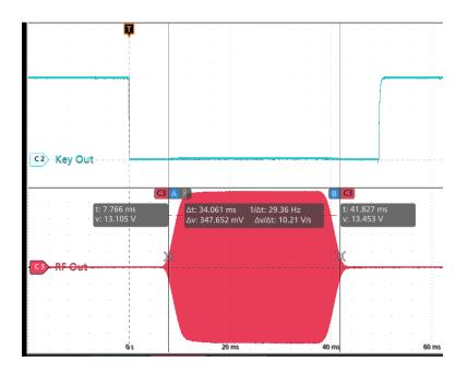
Figure 1 - 8 millisecond Transmit Delay
