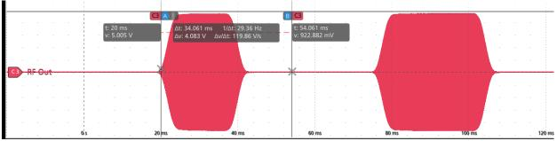
Figure 6 - Increasing delay times in the K3 can cause the first dit to be truncated
