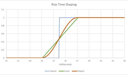
Figure 2 - Pulse shape as well as rise time can reduce clicks.
