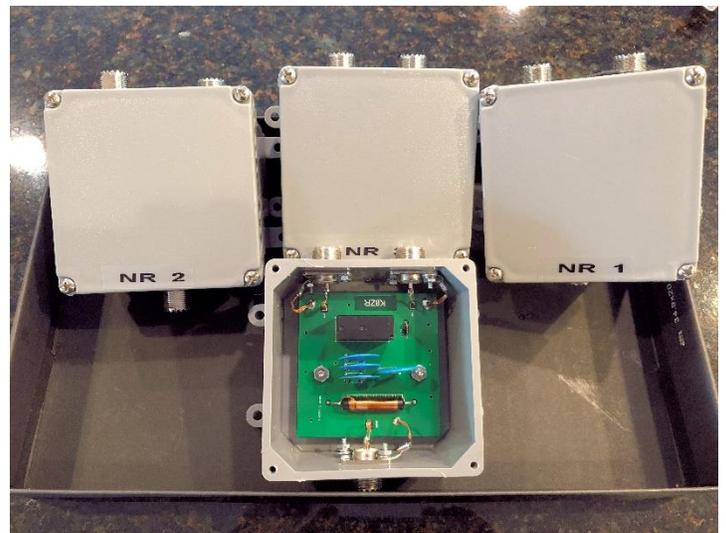
**Figure 12 Four Remote RF Switch Units**
