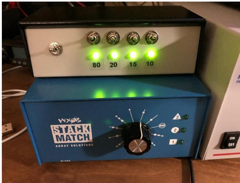
Figure 14 Controller Activating All Four Alternate Antennas
