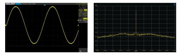
Figure 1: Sine wave (I/h) and its resulting signal in the frequency domain (r/h)
