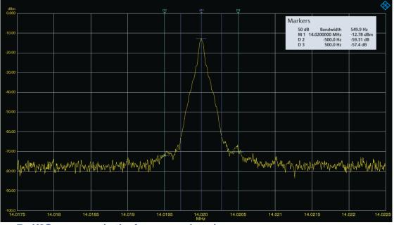
Figure 7: K3S response in the frequency domain
