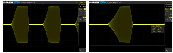
Figure 11: Keying of the IC-7300 at 40 WPM (I/h) and 60 WPM (r/h), using the 8 ms rise time setting (decay remains at 2 ms)
