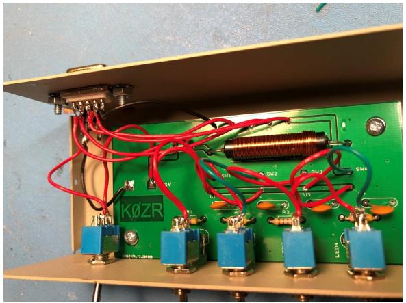
Figure 8 Assembled Controller
