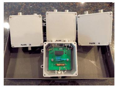
Figure 12 Four Remote RF Switch Units
