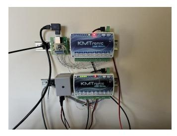
Figure 4 Control switches in shack. Top is RX control, bottom is other antennas
