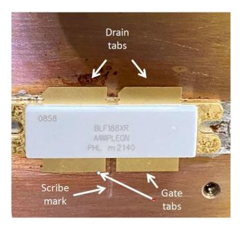
Figure 3 - BLF188XR on heat spreader
