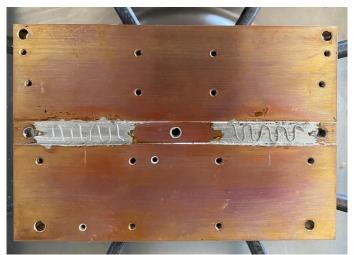
Figure 2 - heat spreader with old solder removed, new solder in the trench
