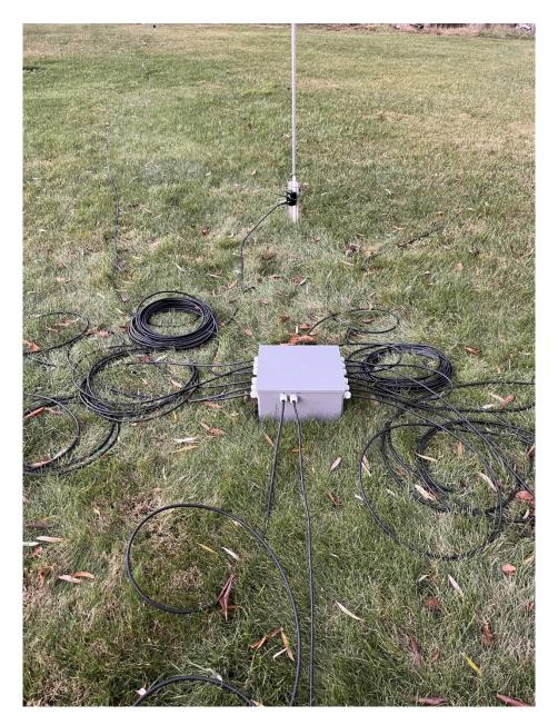
Figure 3. Combiner deployed, coax and center element.
