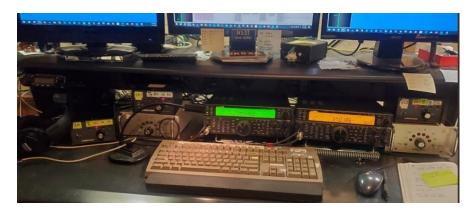
**Jamie NS3T** -I use a three monitor setup for contesting (you can only see the bottom of each monitor in the picture). I have a pair of TS-590SG rigs; I set the radios so that each one has a different color background. Each one has ICE-419A filters for SO2R operations. I also have remote antenna boxes for various bands on the shack table.
