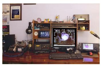
Mike N4CF It shares space with my home office on a 10-foot homemade walnut desk. On the right is an Elecraft K4D transceiver, and in the left hutch bay a KPA500 amp sits on a KAT500 tuner. To the left of the hutch are the main DC power supply, a dummy load, antenna switch, a label printer, and the office computer.
