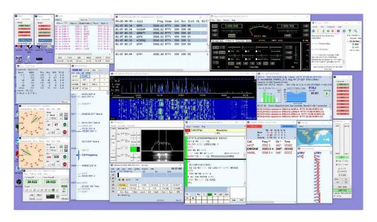
**K3AJ** - a screenshot of what the remote operators see at K3AJ. Not exactly a shack picture - a virtual shack picture! This is all spread over a 27" monitor in the shack. The remote operators use remote desktop software (VNC Server/Viewer) to see and control this display from their computers. This is from a RTTY contest (RTTY RU), so it is especially busy.
