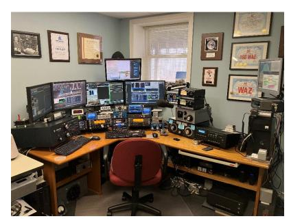
Mark K4SO Ergonomic layout with antenna selection centrally located. SixPak driven (both sides) by decoders on each K3. Easy to do the right parts.
