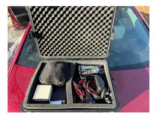
The case on the right is a faux Pelican case that I purchased from Harbor Freight. On the left side is the TS-480 body. The small box is a Signa-Link that I use for digital, I mainly run FT-8 or FT-4. The mesh bag was from a long ago used headset I had for work. That contains all the non-power cables. The right side of the case contains the TS-480 head. On the bottom is a LDG 200 wat auto tuner. I also have the two power
