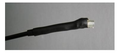
Figure 18. Completed female cable-end connector.
