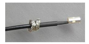
Figure 15. Inner heat-shrink in place.
