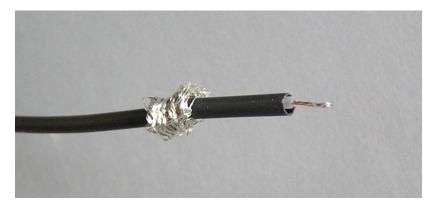
Figure 13. Coax end prepared (inner piece of heat-shrink hidden inside outer piece).
