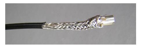
Figure 17. Braid soldered to connector shell.
