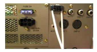
Figure 4. Cables exiting through gaps by the ACC 4 connector.
