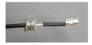
Figure 16. Outer heat-shrink in place.
