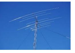
6063-T832 Aluminium TX38 Triband Yagi Antenna 10-15-20 Meter with Monoband Performance 2 Elements on 15 and 20 and 4 Elements on 10 All hardware weather resistant Antenna Rated for over 100 MPH
