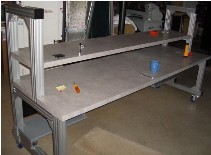
I added two small shelves underneath for power supplies and such. The back wall has dedicated power outlets and a mains filter, all controlled by one master switch on the front leg. In addition, I fabricated some wide aluminum hooks to aid in cable management.
