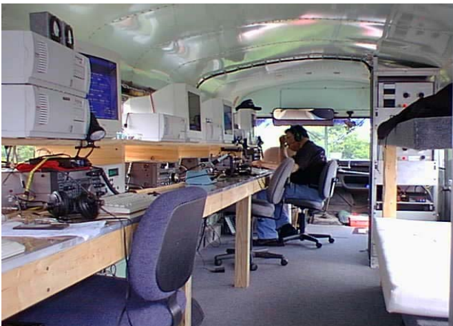
The operating positions from the rear entrance of R2B2. 2304 MHz and above is the nearest position, then 903/1296 MHz, Rover coordination station, 222 MHz and W3ZZ sitting in front of the 432 MHz position.
