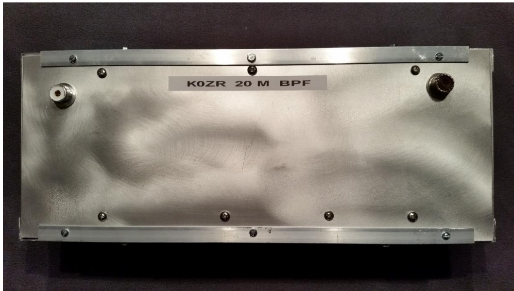
Figure 30 BPF in Homebrew Aluminum Housing
