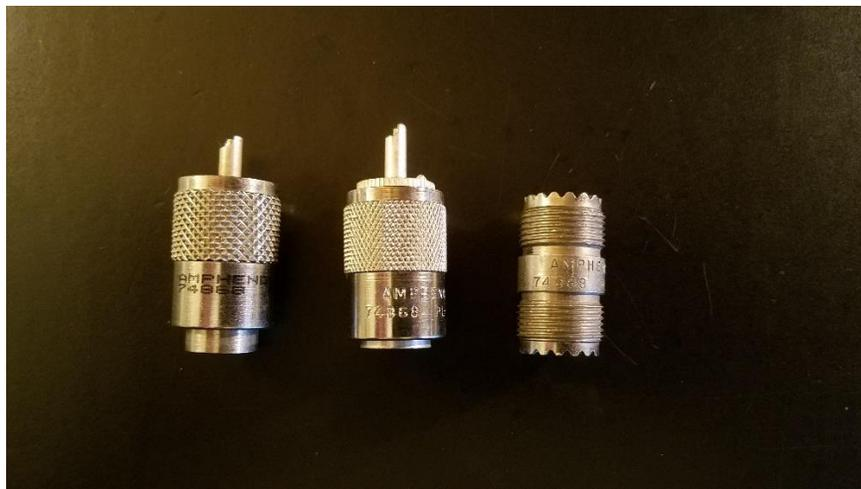
Figure 2. Examples of Amphenol PL-259 connectors. The left one is marked in ink, the center and right one have their markings stamped into the body. All carry both the name of the manufacturer and a part number. The inked PL-259 is an authentic Amphenol.
