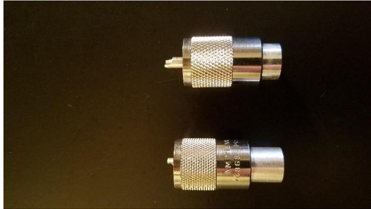
Figure 3. An Amphenol and an unmarked PL-259. The unmarked part was bought from MAX-GAIN and is known to be an excellent product.
