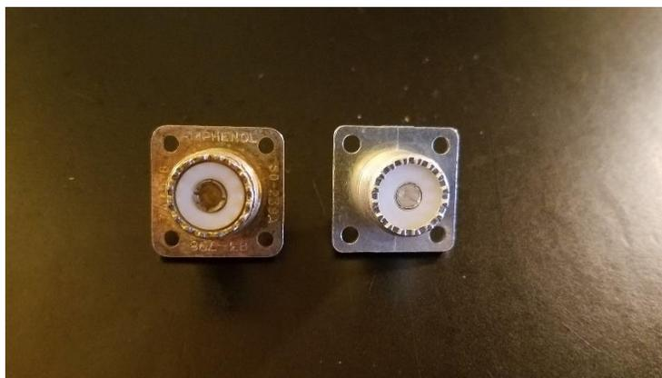
Figure 5. SO-239s. The one on the left is an old Amphenol that is clearly marked. The marks include the manufacturer, the type and the part number – there is zero mystery about what this is. The one on the right is a “mystery” connector. The old Amphenol fits tightly with a PL-259 and is perfectly serviceable. The nice shiny brand new one on the right is junk – a PL-259 slips into it so easily the connection is intermittent.
