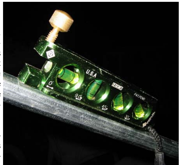
Fig. 1—Greenlee Electrician’s Level
